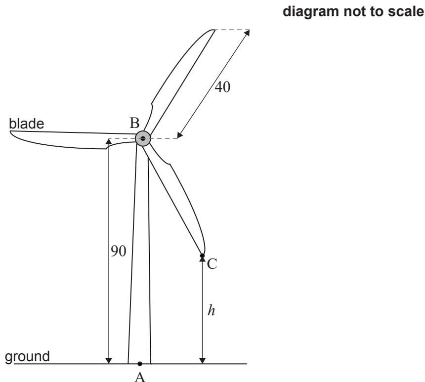
The end of one of the blades of the turbine is represented by point C on the diagram. Let  $h$  be the height of C above the ground, measured in metres, where  $h$  varies as the blade rotates.
